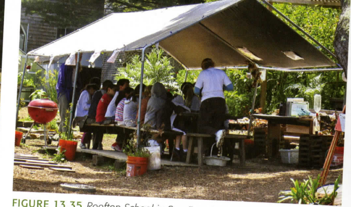
FIGURE 13.35 Rooftop School in San Francisco, California, uses a lightweight canopy to shelter an outdoor teaching space from the sun and light rain. Shelters like this one are intended to be portable, but some are sturdy enough to leave in place for years if the weather is mild.
